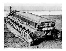
Amphibious Bridge Vehicle (Floats attached, being prepared for water travel; rear wheels are retracked)
